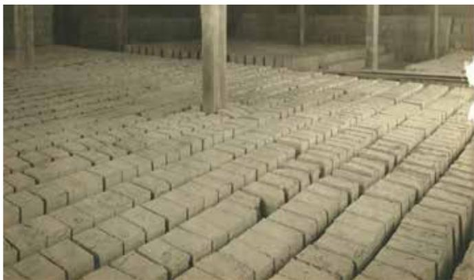
Refractory brick was designed to withstand the high temperatures of the interiors of furnaces, ovens, and locomotive fireboxes. Photo from the Brian K. Fenton Photo Collection.
